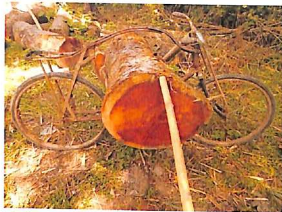
Modified Bicycles used for Transportation of Logs
