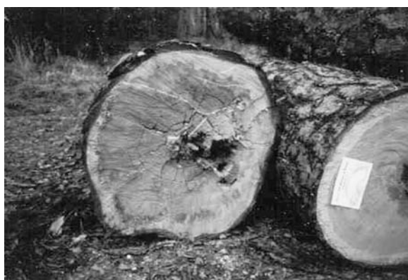
Figure 10.6. Brown rot in the heartwood of a pine tree. The rot started in the living tree.
