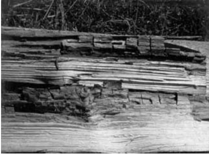
Figure 10.12. Brown rot in pine wood. Note the cubical cracking.
