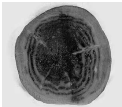
Figure 10.30. Heart rot caused by Phellinus pini in a pine wood tree used to construct the bulwark in lake Tingståde ca 1100 AD. The log has been laying at the bottom of the lake for nearly 900 years. Soft rot attack can be seen as a thin outer blackish layer. Attack by erosion bacteria has occurred to a depth of ca 30–40 mm. Soft rot and bacterial attack occurred while the log was submersed in the lake water.
