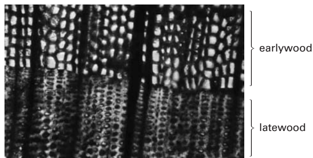
Figure 2.16. The transverse view of the early- and latewood cells in softwood (Scots pine). The difference between the thick walled latewood- and the thin walled earlywood tracheids will be visible in the wood as year rings. Year rings can be formed in other ways in hardwood as discussed in chapter 3.
