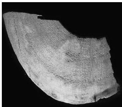
Figure 10.31. Heart rot in the pine wood foremast of the ship Vasa . The tree felled to be used as a mast was already rotten!
