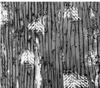
Figure 10.14. Brown rot in pine wood. Only the crossfield pit areas exhibit birefringence (light microscopy, polarized light).
