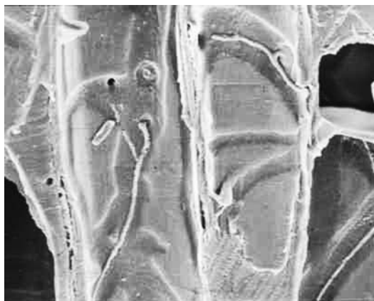
Figure 10.1. Hyphae of the white-rot fungus Phlebiopsis radiata growing in pine tracheids. Note erosion of the tracheid walls along the hyphae. SEM.
