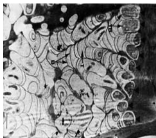
Figure 10.23. Branching tunnels caused by tunnelling bacteria. Note the bacteria at the front of each tunnel (TEM, Courtesy Adya Singh).
