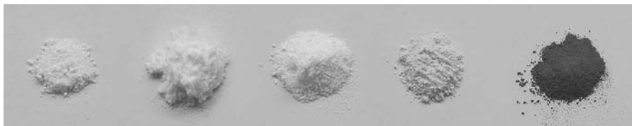
Figure 3.23 Photographs of powders of mesoporous hybrid materials with various conjugated \pi -electron systems (from left to right): ethene-, benzene-, 1,4-divinylbenzene-, 4,4'-divinylstilbene-, and 4,4'-divinylazobenzene-bridged organosilicas. (See color insert.)
