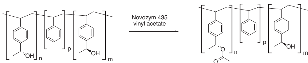
Scheme 11.21 Synthesis of a polymer with two ester groups for enzymatic transesterification and its modification by enzymatic transesterification.
