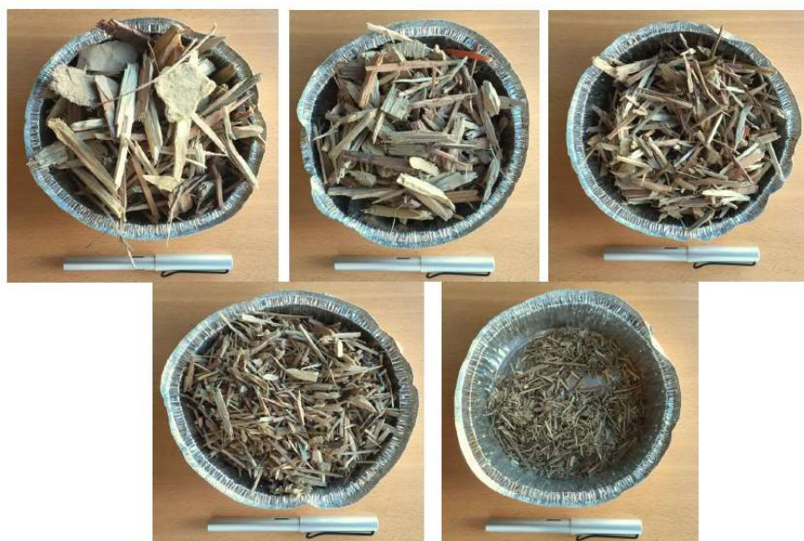
Figure 3. The fuel samples were separated into five sizes. Particle size (x) from the top left to the bottom: x > 25 mm, 12.5 < x < 25 mm, 6.3 < x < 12.5 mm, 3.15 < x < 6.3 mm, and x < 3.15 mm.
