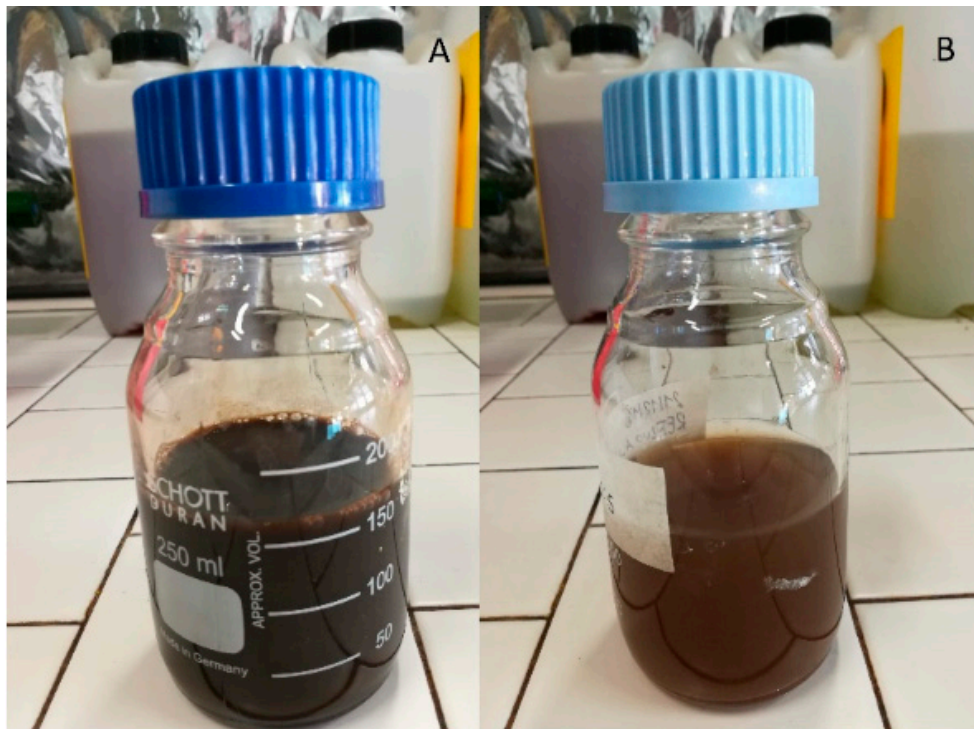
Figure 1. Liquid fraction of digestate from anaerobic digestion of the organic fraction of municipal solid waste (OFMSW): (A) as such; (B) diluted 1:5.
