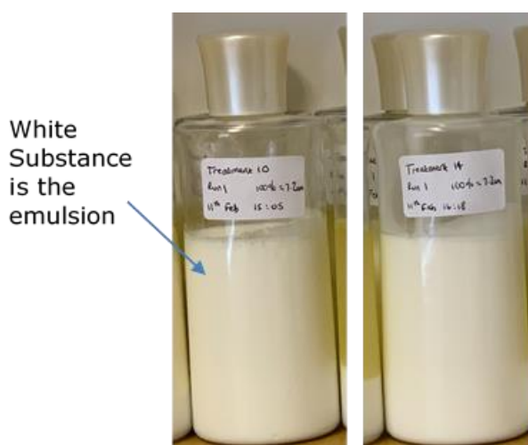
Figure 7. Treatments 10 and 14 displaying 100% stability after 14 days.
