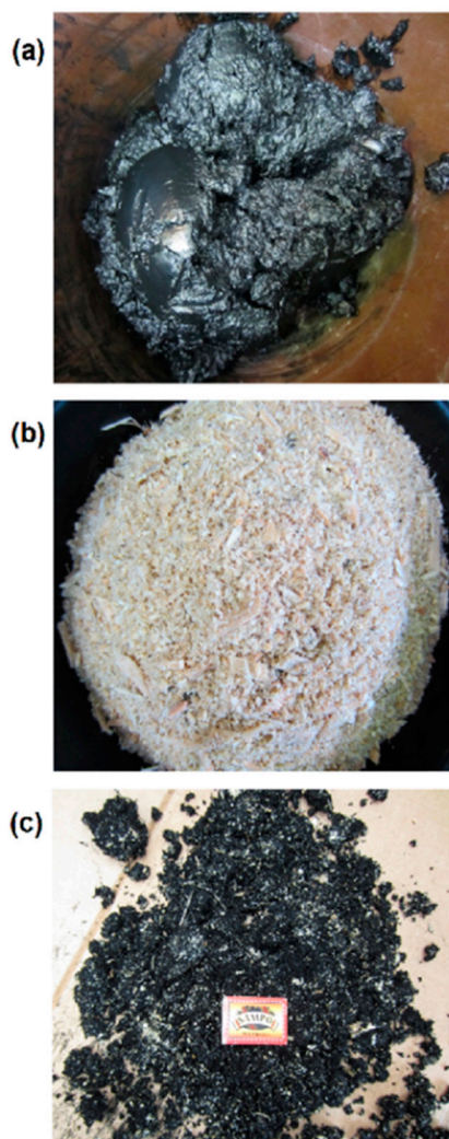
Figure 3. (a) Moist soot sludge (95% wb), (b) moist sawdust (56% wb), (c) moist soot sludge and sawdust mixture (mixture ratio in vol. %: 50% soot sludge and 50% sawdust). (Reproduced from [5]).
