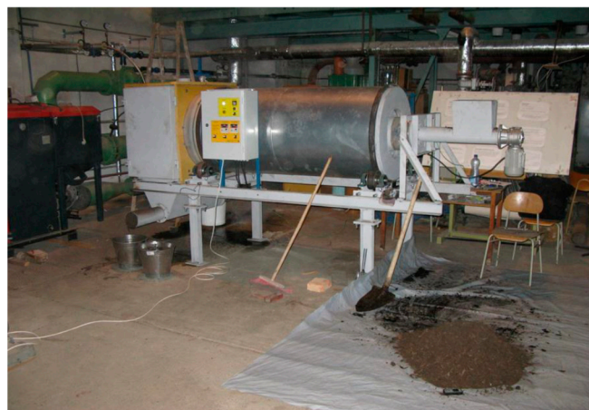
Figure 5. Steam heated rotary dryer.
