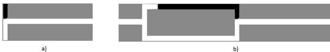
Figure 5. (a) Standard geometry of the T-junction; (b) modified geometry for periodic boundary conditions.
