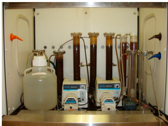
Figure 1. The laboratory facility for the treatment of sucralose production wastewater with recalcitrant organic compounds.
