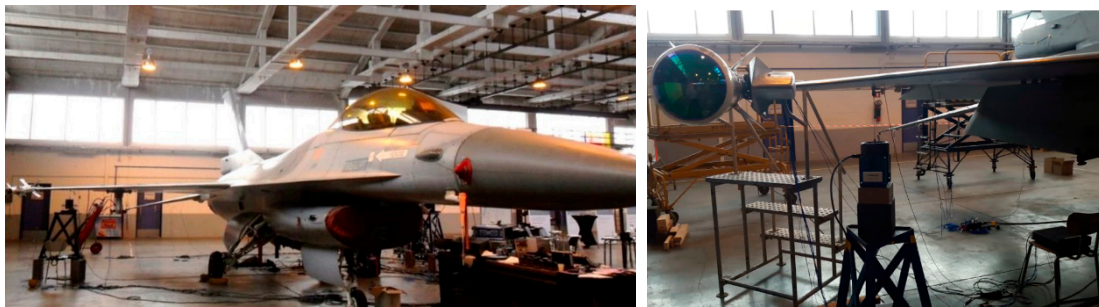
Figure 7. F-16 ground vibration testing measurement campaign. The right wing is excited by a shaker; the voltage (reference) and force (input) signals of the shaker are measured. The major part of the nonlinearities is related to the payload connection interface where the acceleration is measured.
