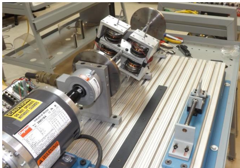
Figure 15. Image of the experimental setup with the ATTVA mounted in the activated configuration.
