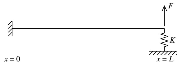
Figure 4. Sketch of the mechanical model, with a stretched string terminated in a spring representing the transducer stiffness.
