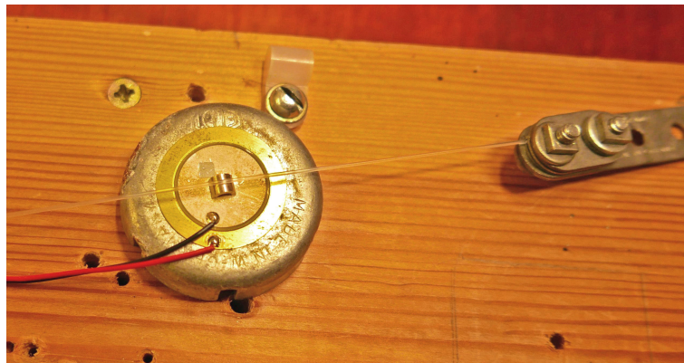
Figure 2. The piezoelectric transducer sitting on top of its circular support. The string is held away from the transducer and support with a semi-cylindrical steel spacer, with a mass of about 0.2 g. The main string section enters from the left of the picture, while the tail section and end clamp are to the right of the transducer assembly.
